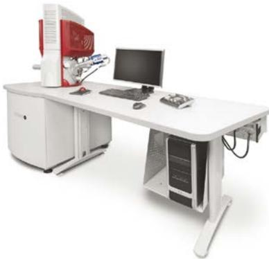
The [Tescan Mira3](#) Scanning Electron Microscopy is used for imaging and analyzing the microstructures of materials. The Mira SEM can image structures less than 10 nm in size and can work at low beam voltages meaning materials that can be damaged by higher voltages typically used in SEMs can be imaged without destroying them. The Mira is equipped with Energy-dispersive spectroscopy (EDS) is a small probe analytical technique that can identify elements in a sample down to the submicron scale.
