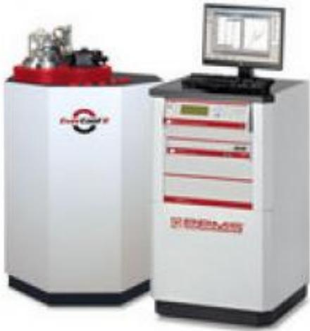
[Quantum Design Physical Property Measurement System](#) is available for magnetic moment vs. field (M vs. H) measurements at room temperature using a vibrating sample magnetometer (VSM). The instrument is also capable of performing a variety of magnetic, electronic transport, and thermal transport measurements under a wide range of temperatures and magnetic fields.
