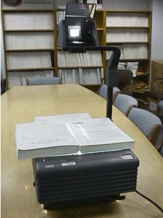
Set-up for the experiment, including the overhead, books to create a slit of light, and the diffraction grating (at top of overhead)
