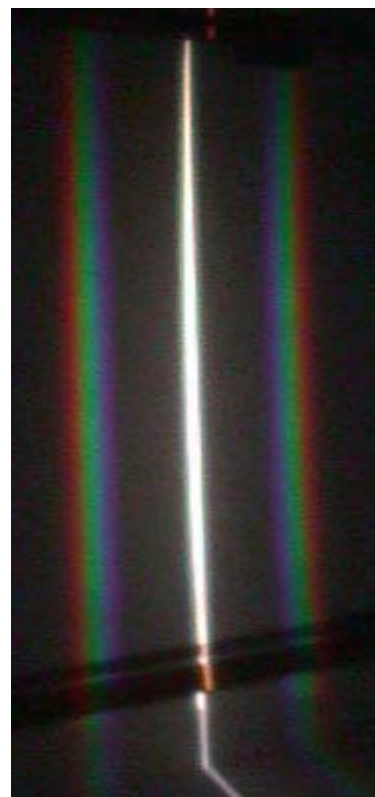
The image on the screen shows the central white band of light coming from the projector, plus a spectrum on both sides.
