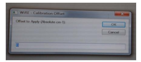
Take the spectrum again to make sure the peak is now close to 520 cm-1. When it is close, then run Quick Calibration again and the offset will be adjusted automatically to put the peak as close to 520 cm-1 as possible.
