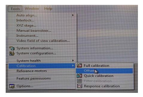
This will open up the window shown below. Enter an offset that will correct for the amount that the Si peak is displaced from 520 cm-1.
