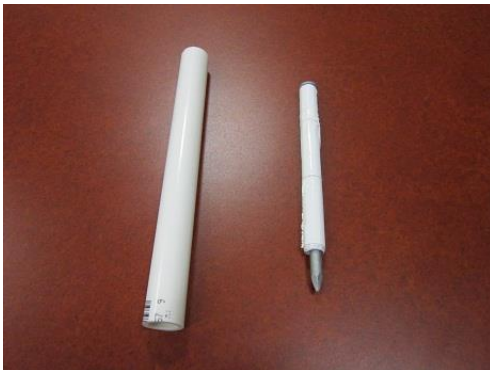
PVC pipe and wrapped nail
