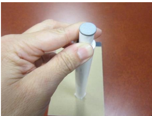
PVC pipe and wrapped nail
