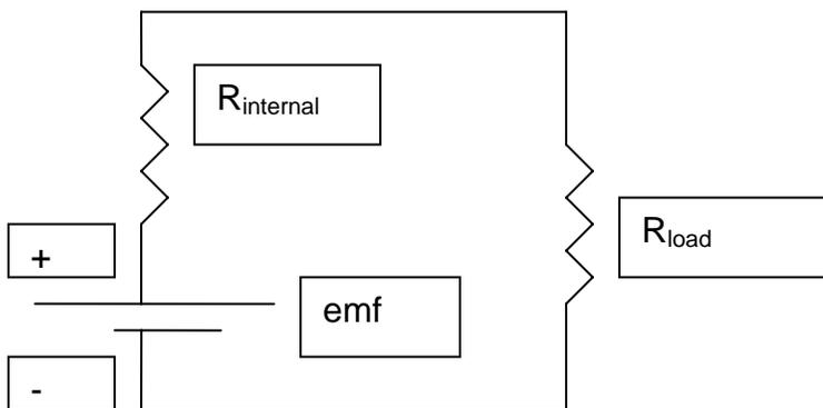
The solar cell is modeled as a voltage (emf) source connected in series with an “internal” resistance. The emf of the cell may be determined by placing a voltmeter in parallel between the terminals of the open circuit. To determine the maximum current of the cell, place an ammeter in series with an otherwise short circuit. It is then possible to define the “internal resistance” of the cell using Ohm’s Law.
