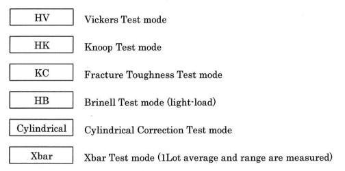
[TEST] is select from [Main Menu] when the test mode is changed.
