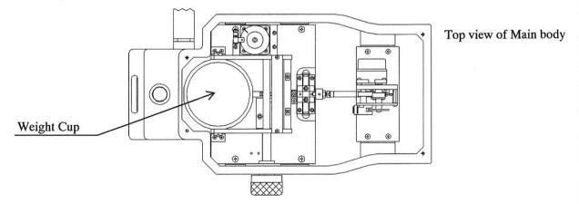
(7) Move the Load Selector Knob from Min. to Max. from Max. to Min. several times. See if the weight cup goes up and down smoothly.
