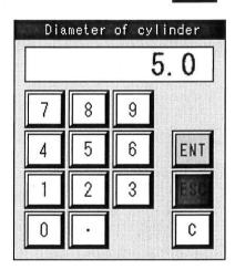
Input diameter, and press an "ENT key".
