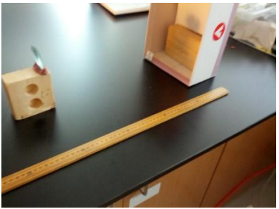
Third lens and screen for image (placed in shoebox to reduce stray light)
