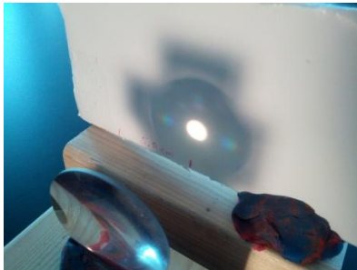
Image of diffraction pattern from grating, produced in focal plane of second lens
