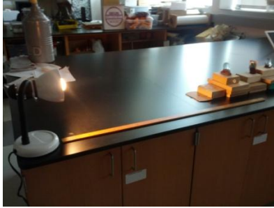
Light source, first lens, 35 mm slide, and second lens
