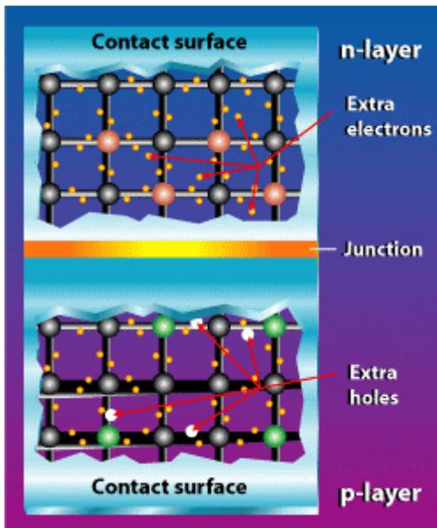
Although both materials are electrically neutral, n-type silicon has excess electrons and p-type silicon has excess holes. Sandwiching these together creates a p/n junction at their interface, thereby creating an electric field.<sup>8</sup>
