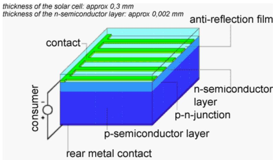
model of a crystalline solar cell<sup>9</sup>
