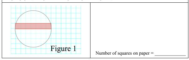
Put the grid paper back at the end of your microscope and look at it again through the microscope with the lenses in the best positions you just determined. Count the number of grid squares you can see across the field of view while looking the microscope in the same way you did above. How many grid squares do you see through the microscope?
