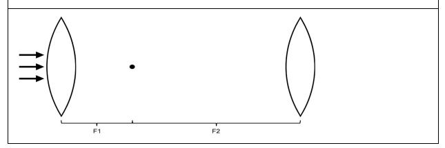
You noticed in the last activity that one lens can be used to magnify an object (like a magnifying glass!). This is known as a simple microscope. A **compound microscope** uses
