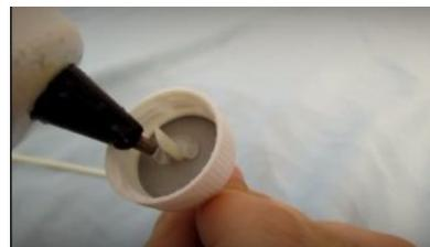
change the bottle size and test the results. Take off the bottle cap and poke a hole in the lid with a nail. Put the lid back on. Insert a 20 foot length of tubing into the hole made in the bottle cap. Seal the edges where the tubing connects carefully with hot glue. Poke a hole
