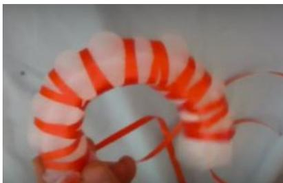
effects of you squeeze the "power source" plastic bottle the pressurized air should move from the squeeze bottle to the robot body and inflate it. Practice squeezing and inflating the body and using it as a gripper. As the robot body deflates, the gripper will grasp the object. Because of the "give" of the soft robot body, the robot should grab the object as it deflating. After the ribbon is wrapped correctly, you
