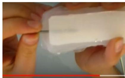
other end of the tubing into the robot body. Glue a piece of duct tape or another molded, thin piece of rubber to the bottom of the gripper to increase its traction and thus its grip.
