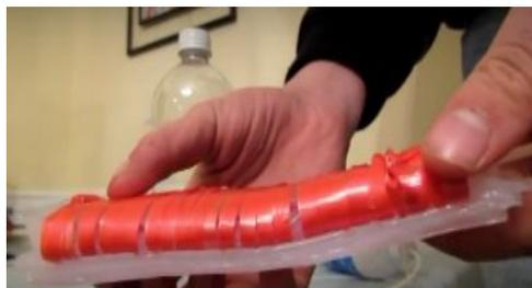
will glue another piece of thin rubber that you have molded for this purpose or a piece of tape to the back of the robot for more gripping traction. One of the most important properties of soft robots is in how they deform while being used. In the case of the soft robot that we build, the robot is powered and moves by the inflation and deflation of the robot body which is its actuator.
