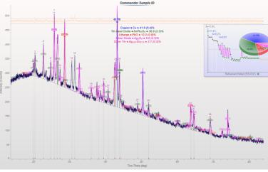
Diffraction patterns and analysis from two different submillimeter areas of whole circuit board, showing material composition of edge connector (left) and solder (right).
