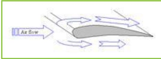
The difference in the speed of the air, combined with the turning of the air downward mean that there is a pressure difference between the top and bottom surface of the wing: there is low pressure on the top of the wing and high pressure underneath the wing. Since objects naturally move toward areas of low pressure, this causes the wing to be 'sucked up' into the air, in an effect called **lift**.
