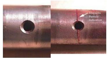
the surface. Iron particles are attracted and concentrated at sites of the magnetic flux leakages. This produces a visible indication of defect on the surface of the material. The images above demonstrate a component before and after inspection using dry magnetic particles.
