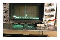
In ultrasonic testing, high-frequency sound waves are transmitted into a material to detect imperfections or to locate changes in material properties. The most commonly used ultrasonic testing technique is pulse echo, whereby sound is introduced into a test object and reflections (echoes) from internal imperfections or the part's geometrical surfaces are returned to a receiver. Below is an example of shear wave weld inspection. Notice the indication extending to the upper limits of
