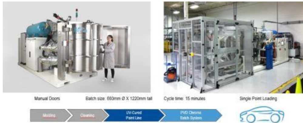
Figure 4 - PVD chromium in industrial production.
