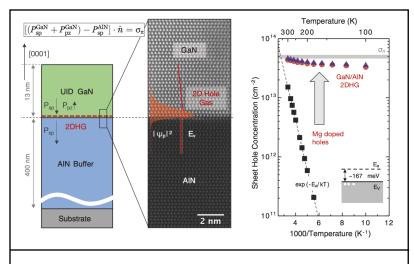
Difference in internal polarization fields at the metalpolar GaN/AIN interface (shown above) gives rise to a negative sheet charge, which induces a layer of mobile positive holes– no chemical impurity doping is required. The resulting holes maintain their high densities at temperatures down to 10 degrees above absolute zero.
