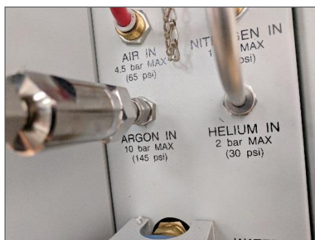
Figure 74: Service Panel Helium Input Connector Before and After Connecting 6 mm Metal Helium Line
